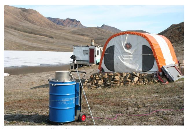
The WiseAsh is a portable, multipurpose batch load incinerator for remote locations, mining camps, job sites, oil drilling operations, truck stops, construction sites, islands, barges, campsites and military installations. Waste materials are loaded into a drum, once ignited the lid is placed on the drum and a whirlwind of fire is created by the high velocity blowers creating a clean combustion.
